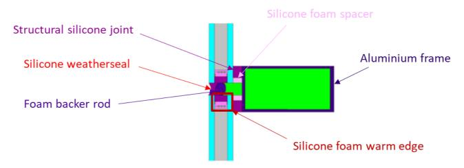
*Figure 14: Silicone structural glazed system*<sup>158</sup>
