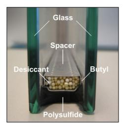
Figure 17: IG unit (section)<sup>189</sup>
