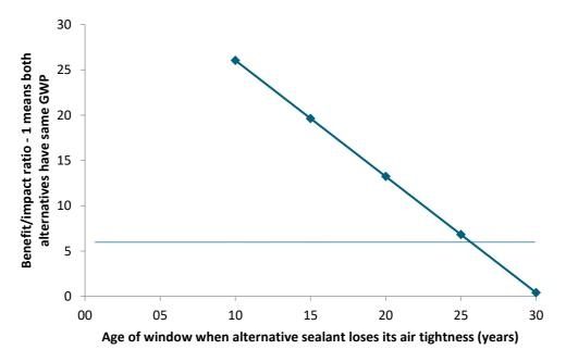
Figure 18: Benefit/impact ratio depending on the assumed lifetime of polysulfide sealant; The horizontal line shows the breakeven point at about 25,5 years.
