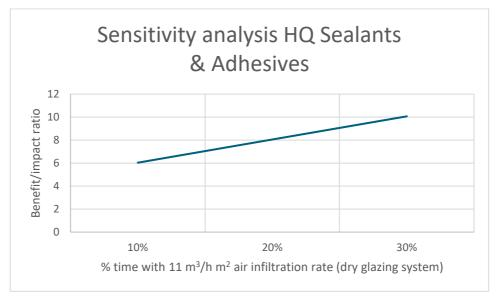
Figure 15: Sensitivity analysis of % of time with 11  $m^3/h$   $m^2$  for the dry glazing system
