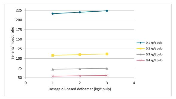
Figure 16: Dependency of benefit/impact ratio on the dosage levels of silicone defoamer and its alternative, oil-based defoamer.
