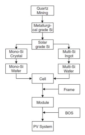
Figure 10: Detailed flow diagram from the raw material acquisition to manufacturing stage of PVs (ds modified from Fthenakis, V.M., Kim, H.C., Alsema, E. (2008)<sup>112</sup>)
