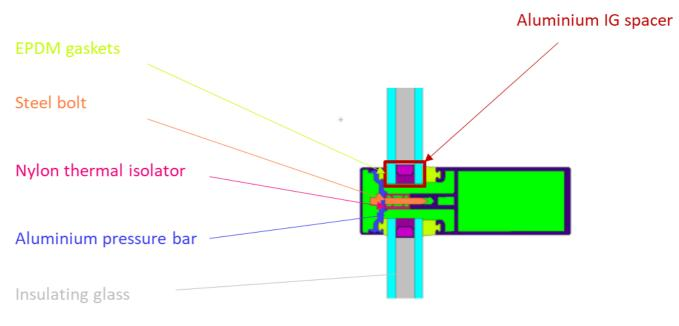
Figure 13: Dry glazed thermally improved system<sup>157</sup>
