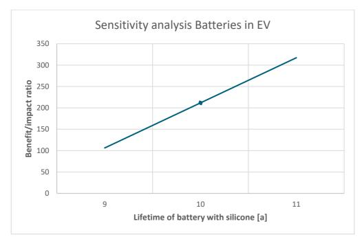
Figure 9: Sensitivity analysis: Batteries in EVs, silicone and epoxy as a Thermal Interface Material
