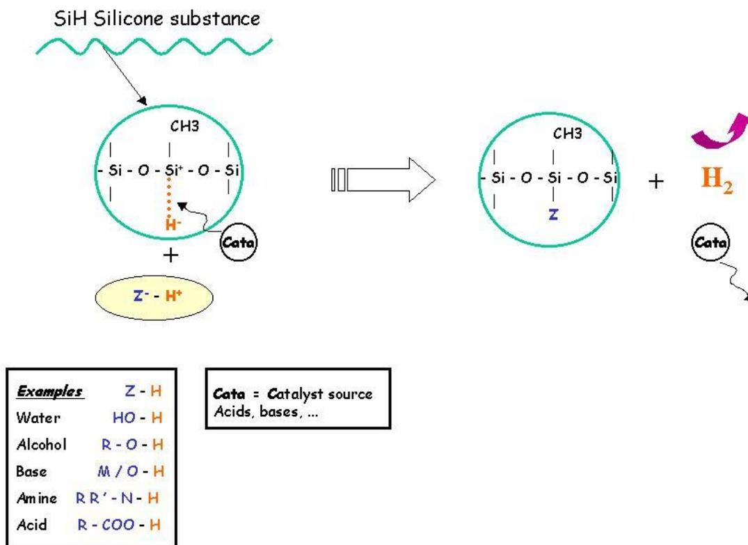
FIG. 1—Gassing Phenomenon of SiH Products.
